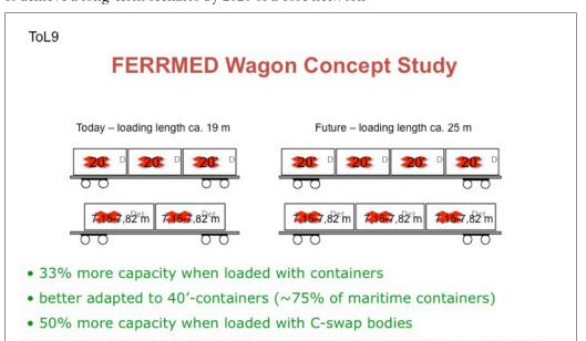
• frame slightly heavier due to longer span, but bigger distance between bogies  $\rightarrow$  tare weight per meter less than today's wagons
