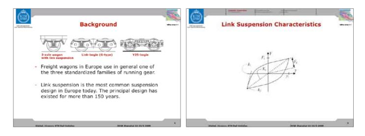
the characteristics. Substantial improvements by means of additional hydraulic dampers have been suggested and tested on modified two- and four-axled wagons on track. Speeds up to 170 km/h have been tested.
