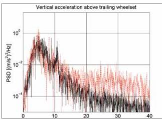
Comparison between measured and simulated results... ... for two-axle vehicle with link suspension.
