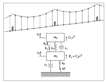
Modelling pantograph catenary interaction with ANSYS.
