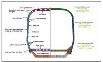
Cross-section comparison between original steel body (left) and a sandwich alternative (right). Number of parts reduced by over 90% for sandwich alternative.
