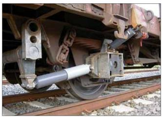
A two-axle wagon with different damper arrangements was successfully tested at speeds up to 176 km/h.
