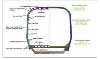
Cross-section comparison between original steel body (left) and a sandwich alternative (right). Number of parts reduced by over 90% for sandwich alternative.
