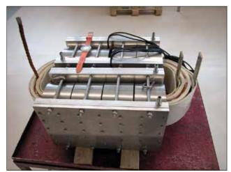
Protoype of medium frequency transformer for 200 kVA, 4 kHz.
