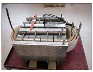
Protoype of medium frequency transformer for 200 kVA, 4 kHz.
