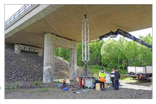
Pilot testing of a hydraulic bridge exciter developed by KTH.
