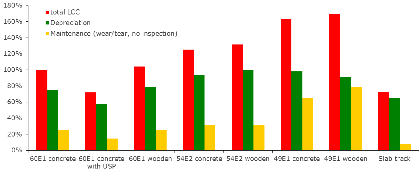
Composition of normalised annual Costs Influence of Superstructure High-loaded, straight Track with good subsoil
