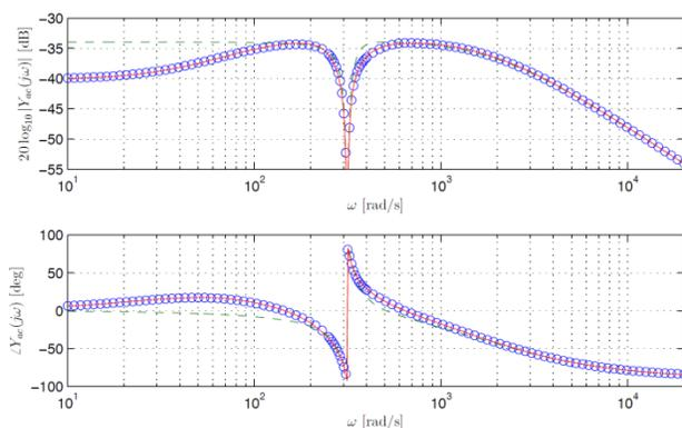
Figure 2: ac/dc MMC input admittance
