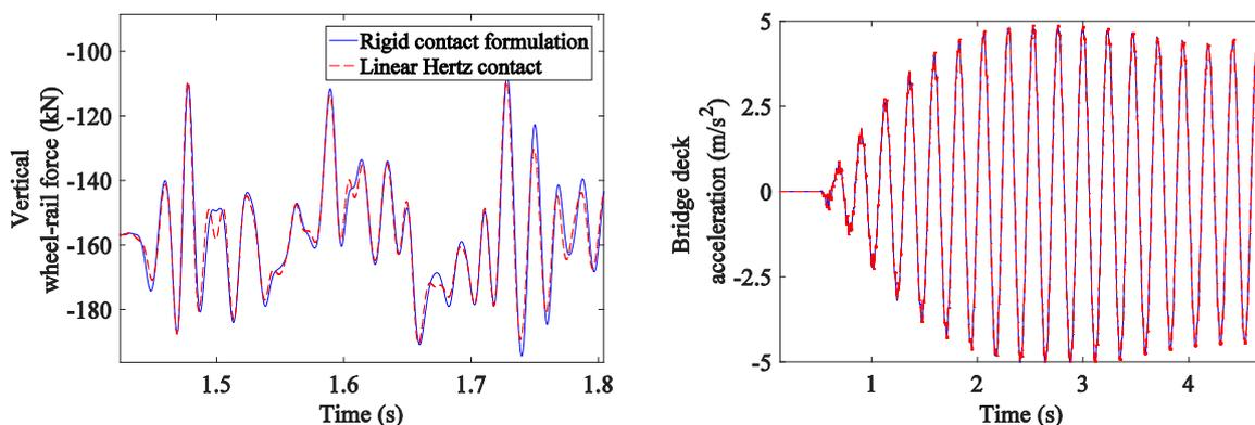
Figure 2. Wheel-rail contact force (left) and bridge deck acceleration (right).
