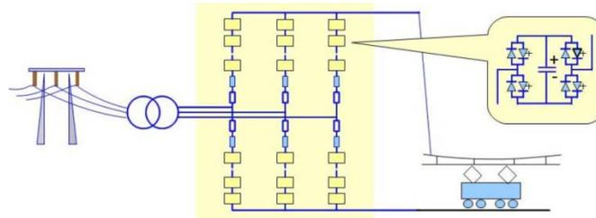
Figure 1: modular multilevel converter for railway application
