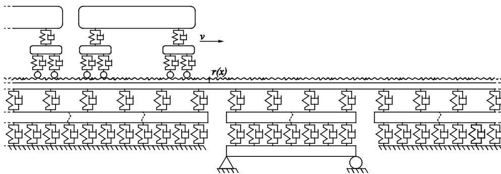
Figure 1. 2D train-track-bridge model for bridges with slab track.
